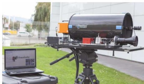
Figure 2: Stand-off detection system based on imaging MIR backscattering spectroscopy, using EC-QCLs for wavelength-selective illumination of the scene to be investigated.
