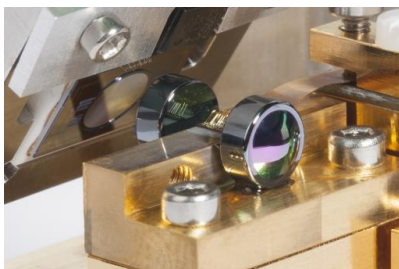
Figure 1: Photograph of an EC-QCL module employing a MOEMS scanning grating in Littrow-configuration as wavelength-selective optical feedback element.
