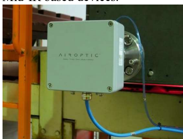
Fig. 1: GasEye in-situ cross duct sensor for low ppb formaldehyde monitoring
