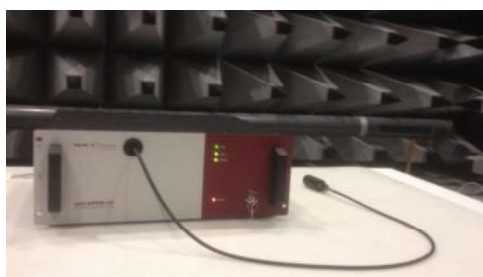
Figure 1: Fully packaged, high repetition rate turnkey mid-IR supercontinuum system from NKT Photonics.
