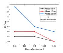
Figure 2. Threshold current Ith vs thickness of upper cladding for different lasers widths (µm)
