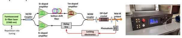
Fig. 1. Experimental setup of the DFG-based comb together with a photo of the prototype of the device.
